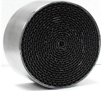
Figure 1.1: Ceramic monolith (up) and catalyst deposition(down left) and
