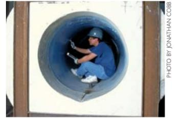
Jie Liu, civil and environmental engineering Ph.D. student, checks for deterioration of concrete coating caused by long-term exposure to various chemicals.
