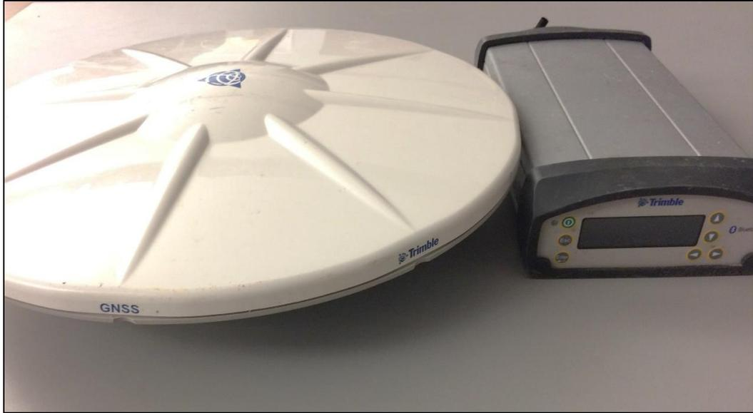
**Fig. 4.4: Trimble Net R9 receiver and Zephyr Geodetic II antenna.** The pair was used for the kinematic GPS survey performed for accuracy assessment purposes.
