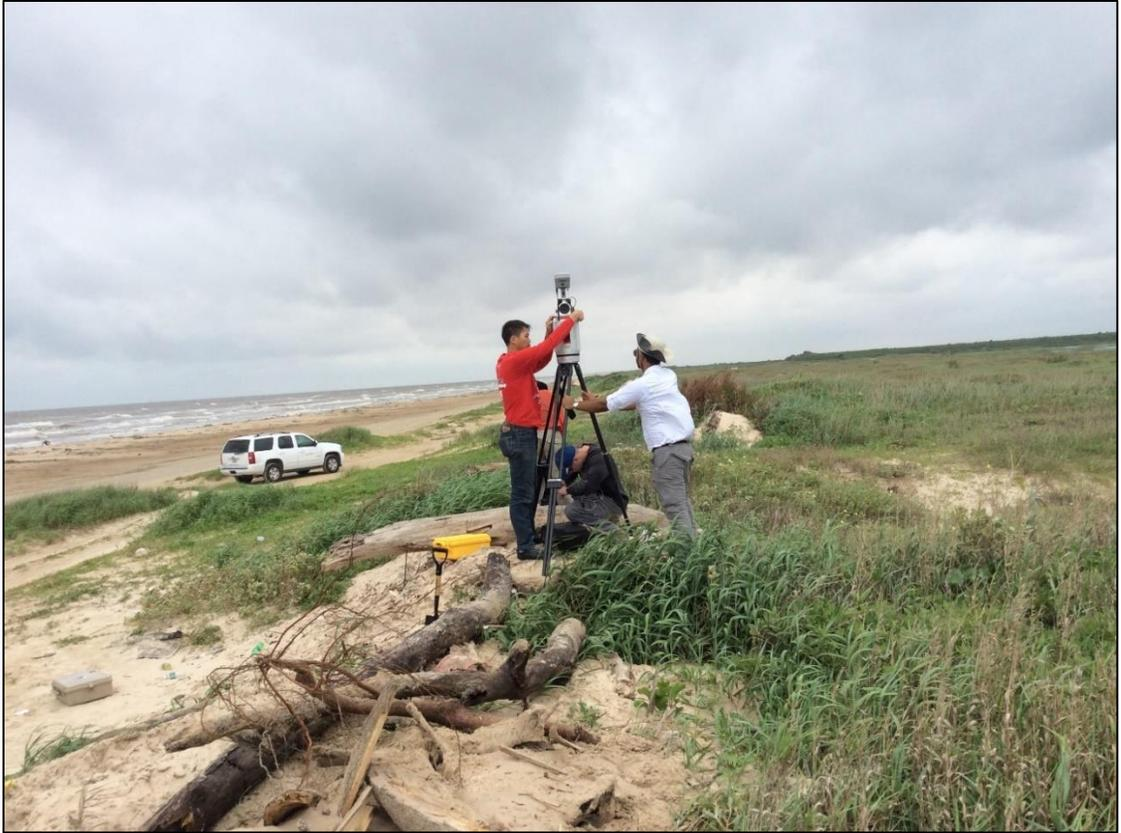
**Fig. 4.11: TLS survey in the coastal area.** The figure depicts the VZ-2000 instrument being mounted on the tripod at a high ground position on the dunes.
