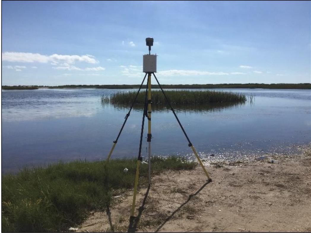
**Fig. 4.5: The reflector or reference point with a GPS unit.** One of the R10 GPS units was mounted on top of a reflector which was used for registration purposes of the TLS datasets.
