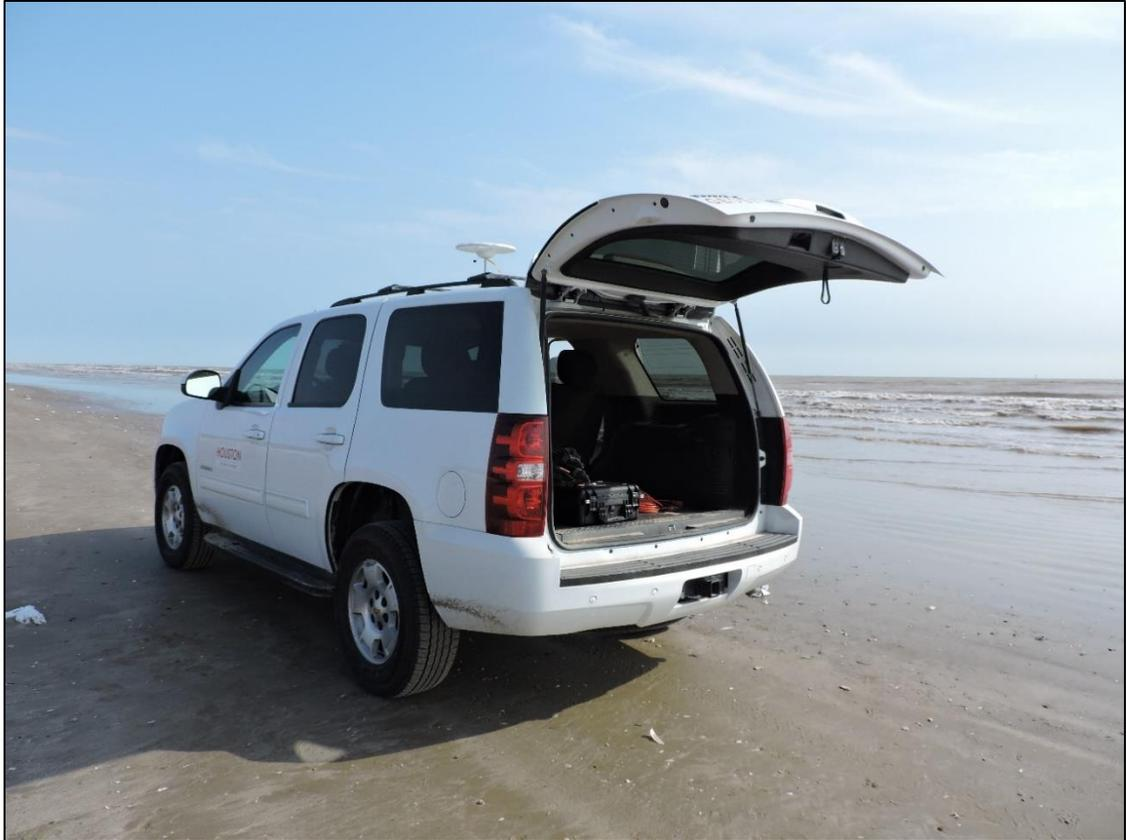
**Fig. 4.8: Kinematic GPS Survey.** The figure shows the car used for the kinematic GPS survey, and the instrument mounted on top. The Zephyr Geodetic II antenna was mounted using a custom-made adapter, while the receiver was kept inside the car.
