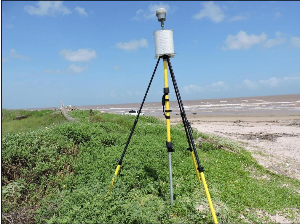
**Fig. 4.6: GPS survey on the dune area.** The reflector points were positioned alternately on the beach area and the dunes.
