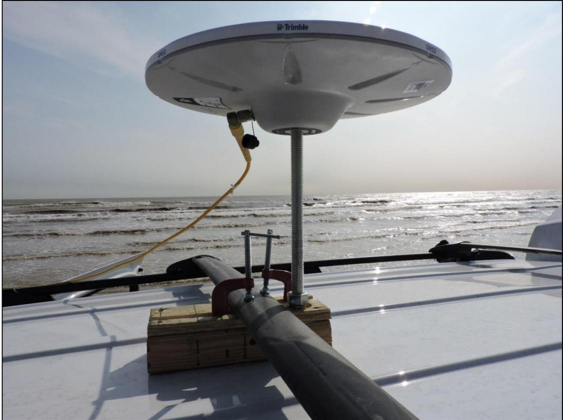
**Fig. 4.9: Antenna used for the kinematic GPS survey.** The picture shows the Zephyr Geodetic II antenna, and the adapter used to mount the antenna on top of the car.
