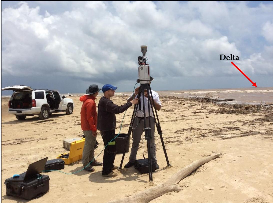
**Fig. 4.10: TLS data acquisition.** The figure above depicts the team collecting TLS data next to the Brazos River delta. The VZ-2000 was mounted on top of a tripod, while the R10 GPS unit was mounted on top of the scanner and the camera.
