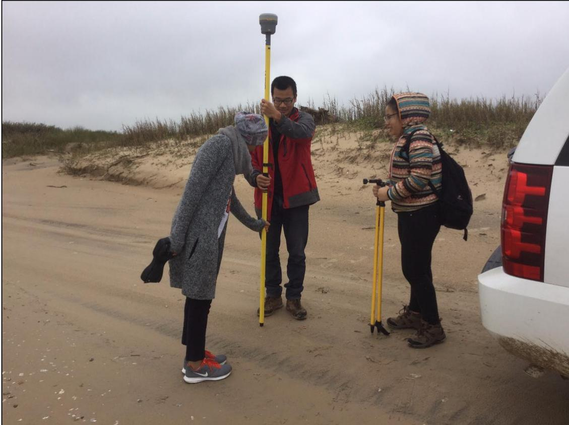
**Fig. 4.7: GPS survey near the dune area.** The R10 GPS unit was used to perform a GPS survey near and through the dunes of the study area.
