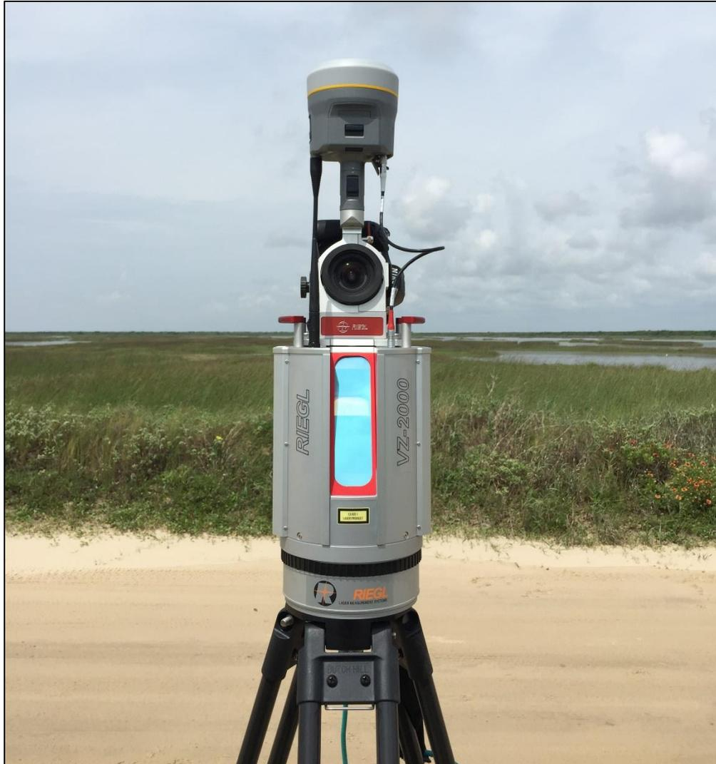
**Fig. 4.1: TLS instrument.** The figure depicts the terrestrial laser scanner used in this study. A VZ-2000 by Riegl company is used with a digital camera and a GPS R10 unit mounted on top.
