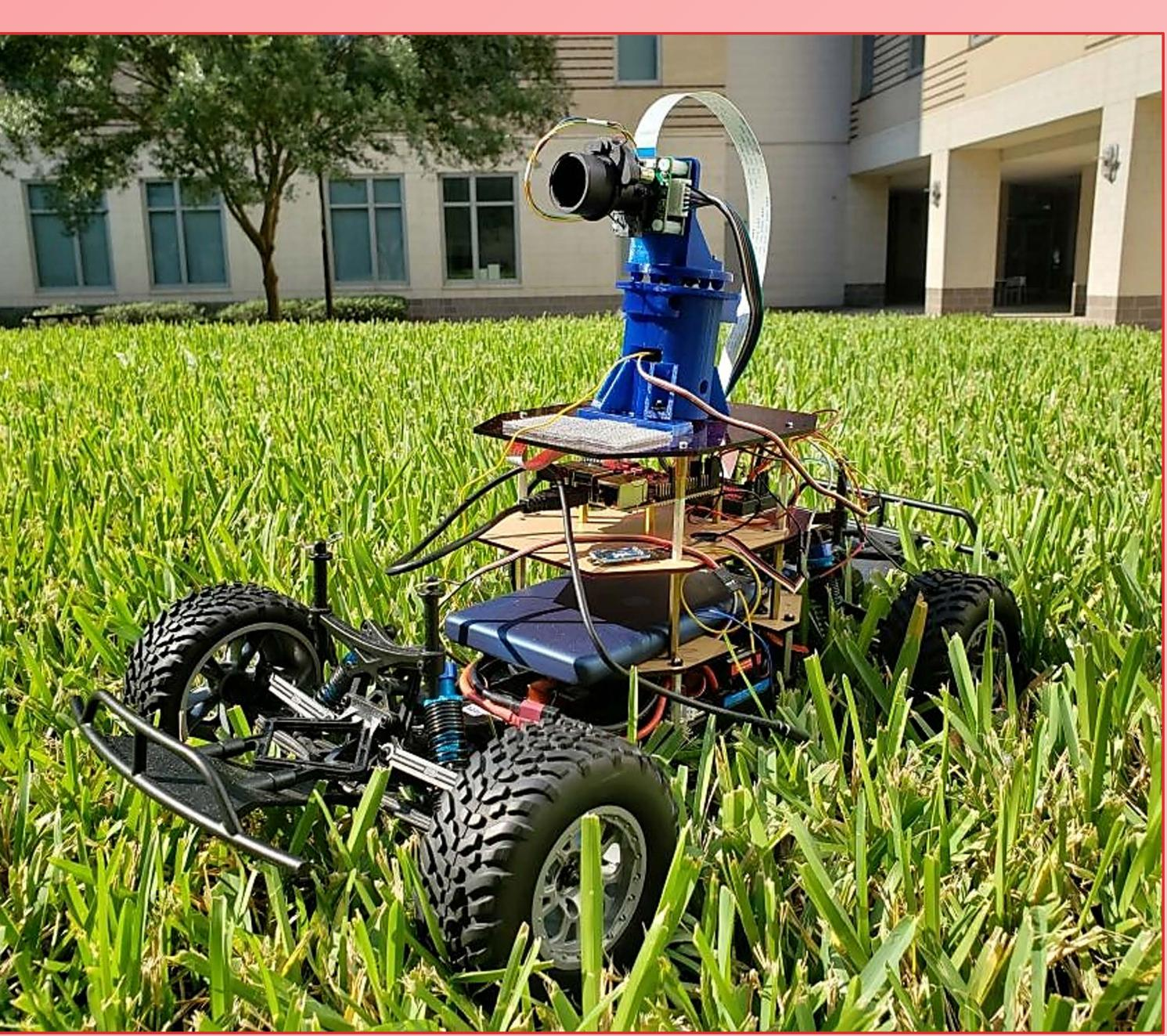
Main body of the robot will be fitted with sensors to interact with its surroundings autonomously.
