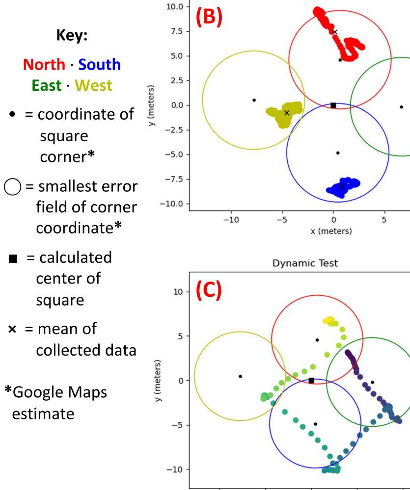
(A) 10m × 10m square plot used to test GPS. Corners marked with red cups; north corner closest to house. (B) GPS data collected at each corner while stationary for 180 second intervals at each corner.
