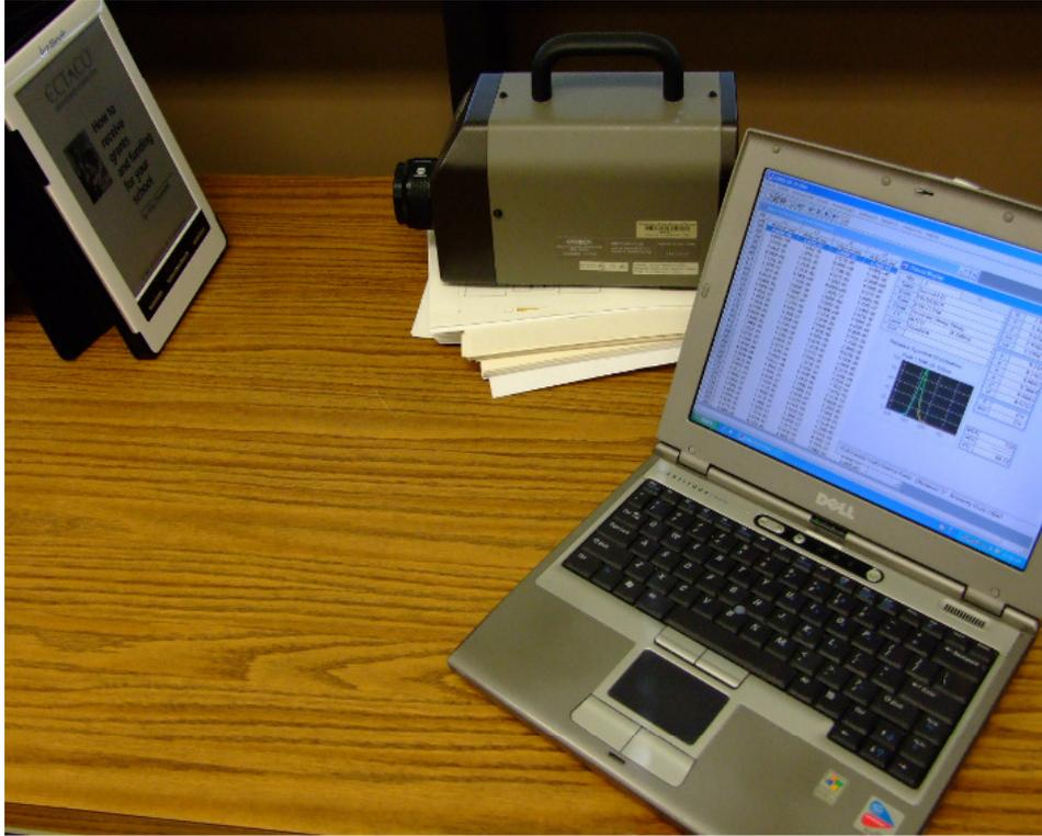
Figure 3.3: Konica Minolta Spectroradiometer and Color EPD
