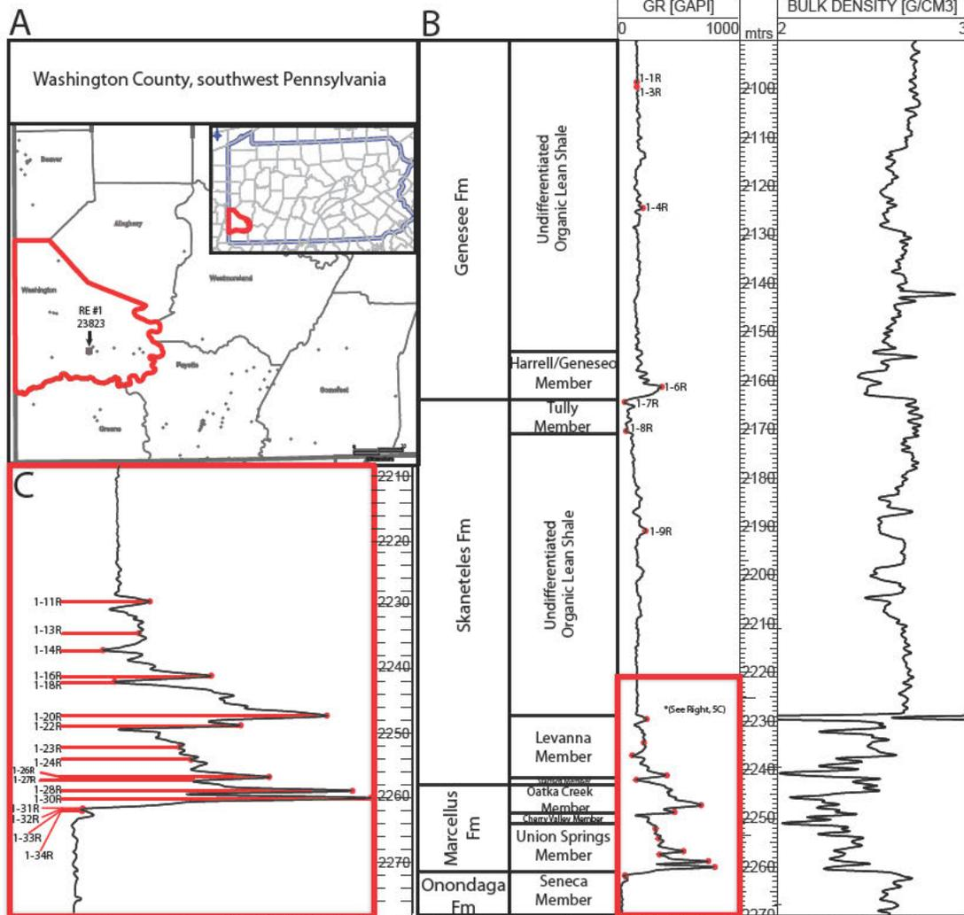
Appendix 1) Location of the RE #1, Washington County, Pennsylvania. **B)** Wireline type log of the RE #1 showing the depth at which each sidewall core was taken and its position relative to the stratigraphic section. Each red dot, on the gamma-ray curve (GR), corresponds to an x-ray diffraction data point as well as a measured TOC (weight %) value. **C)** Gamma-ray curve zoomed-in to the Marcellus Formation.
