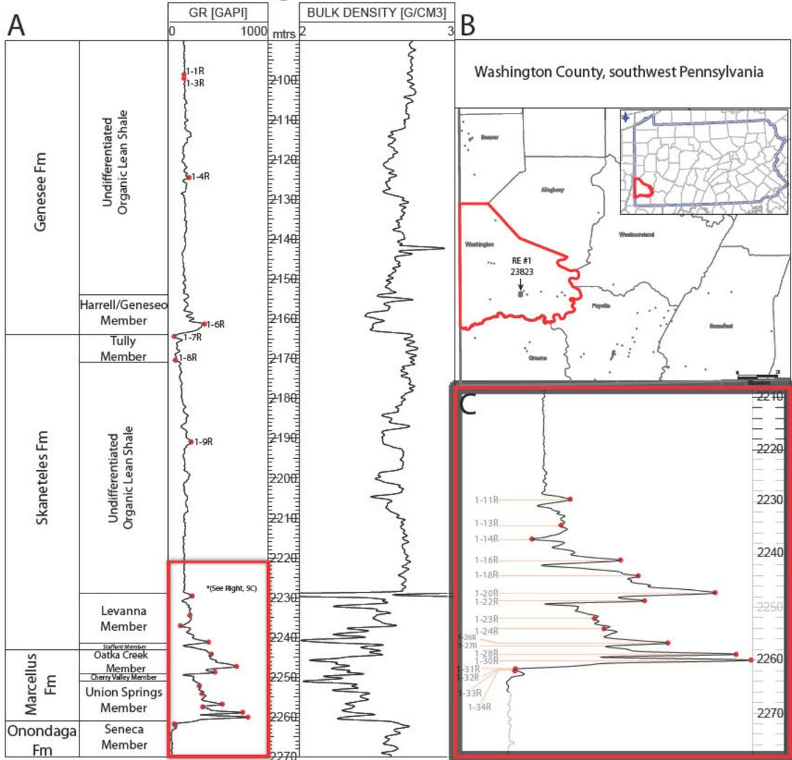
**Figure 5:** **A)** Wireline type log of the RE #1 showing the depth at which each sidewall core was taken and its position relative to the stratigraphic section. Each red dot, on the gamma-ray curve (GR), corresponds to an x-ray diffraction data point as well as a measured TOC (weight %) value. **B)** Location of the RE #1, Washington County, Pennsylvania. **C)** Gamma-ray curve zoomed-in to the Marcellus Formation.
