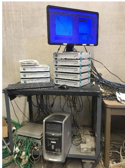
**Fig. 3-7: HBM Spider 8 data acquisition system.**
