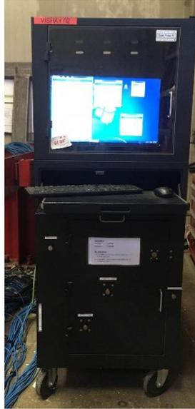
**Fig. 3-8: Vishay data acquisition system.**
