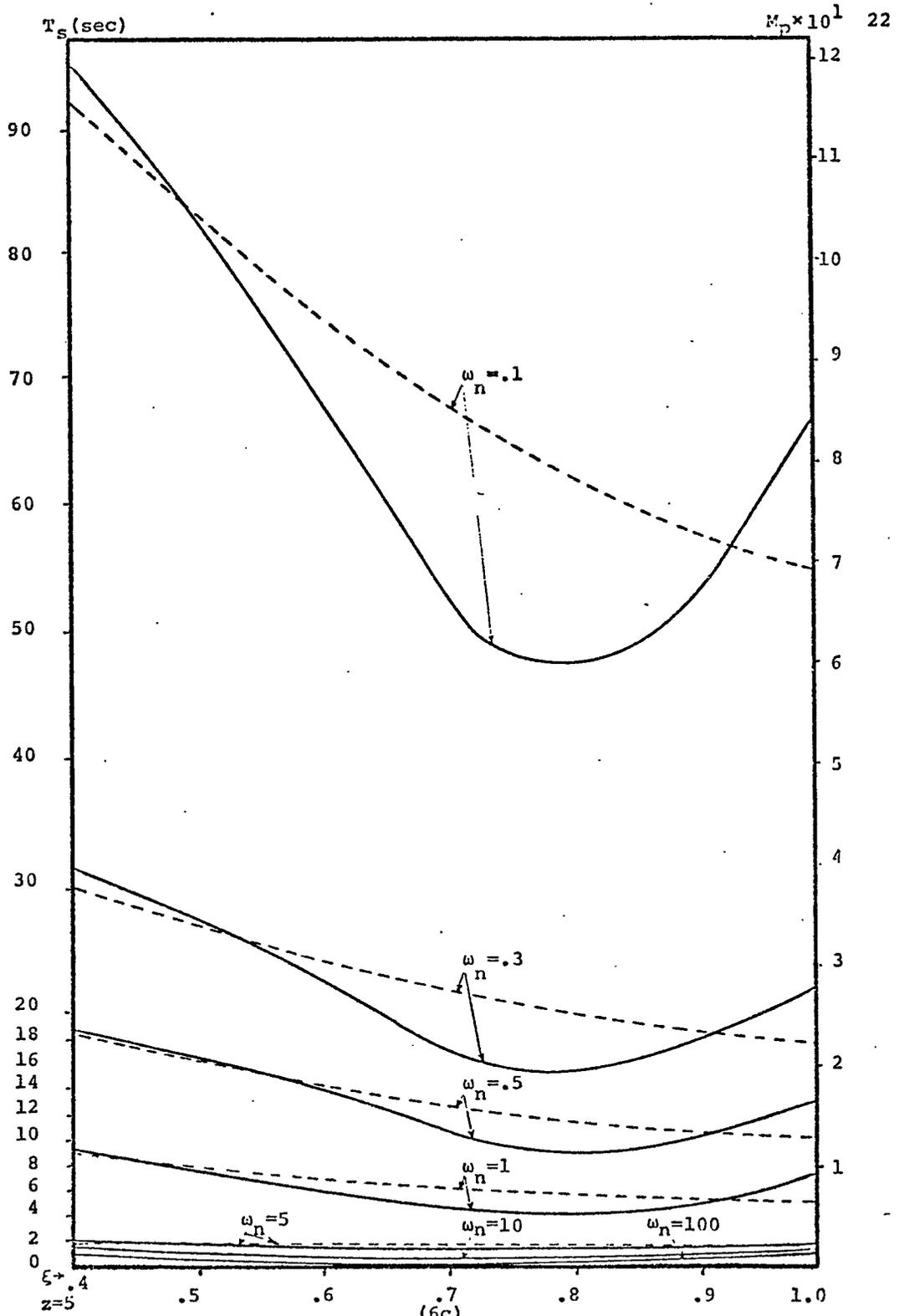
$M_p$  and  $T_s$  of Unit Step Response of Third Order Transfer Function with a Zero at the Origin vs.  $\xi \omega_n$  for  $z=5$
