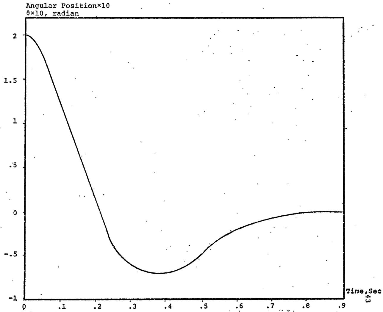
Figure 13. Zero Input Response of the Angular Position for an Initial Angular Position of .2 Radians
