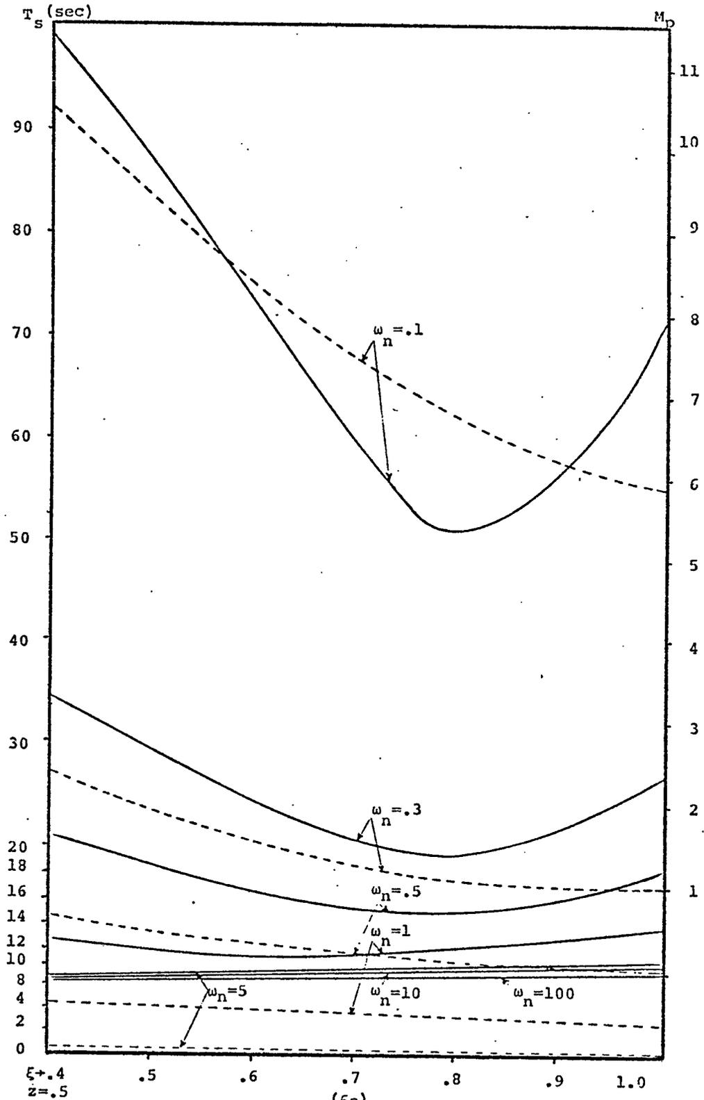
$M_p$  and  $T_s$  of Unit Step Response of Third Order Transfer Function with a Zero at the origin vs.  $\xi\omega_n$  for  $z=.5$
