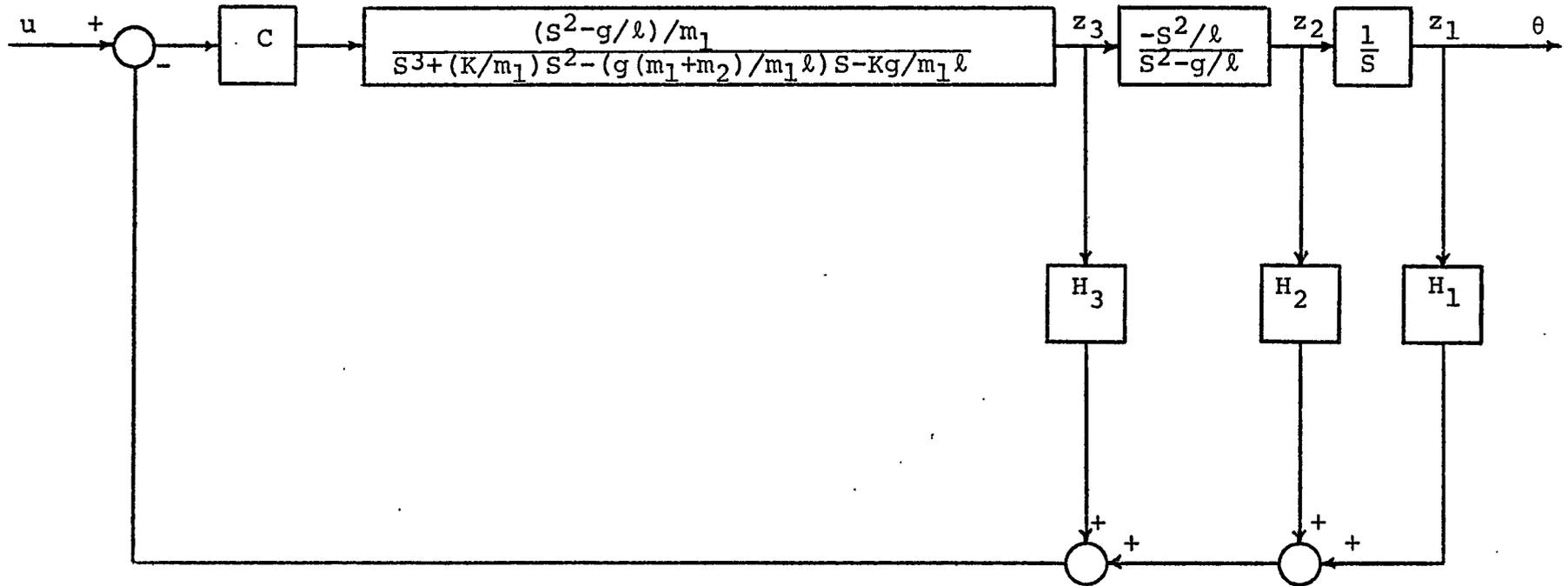
Figure 5. Feedback Control Model of the System
