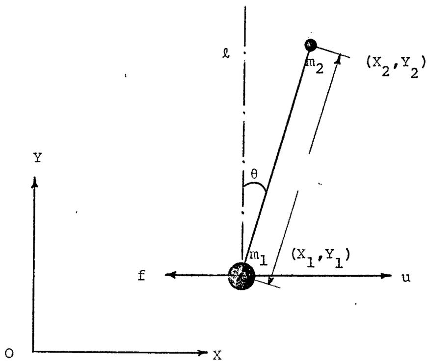
Figure 3. Coordinate System for the Inverted Pendulum
