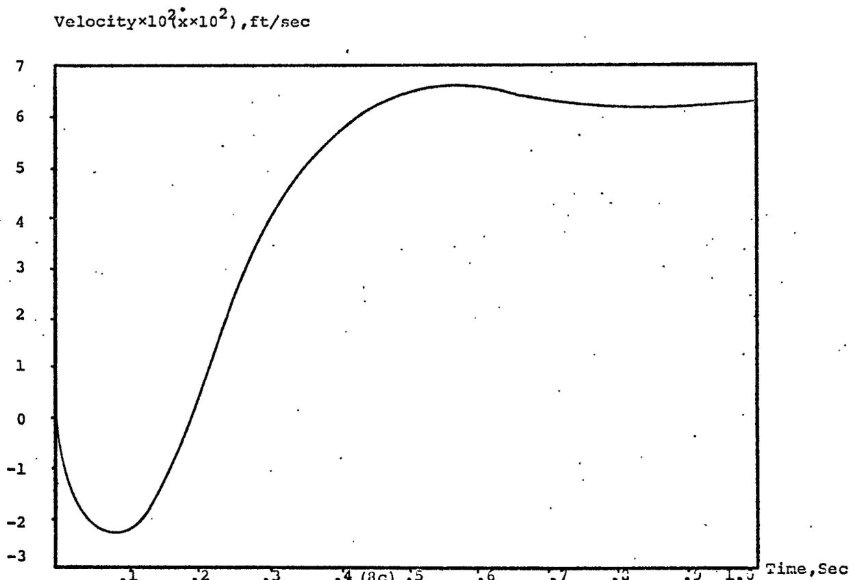
Figure 8. Unit Step Response of the Closed-Loop Nonlinear System
