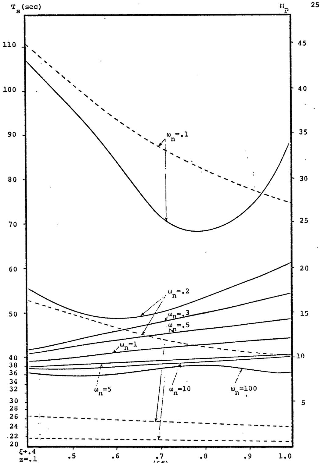
Figure 6.  $M_p$  and  $T_s$  of Unit Step Response of Third Order Transfer Function with a zero at the Origin vs.  $\xi\omega_n$  for Constant  $z$
