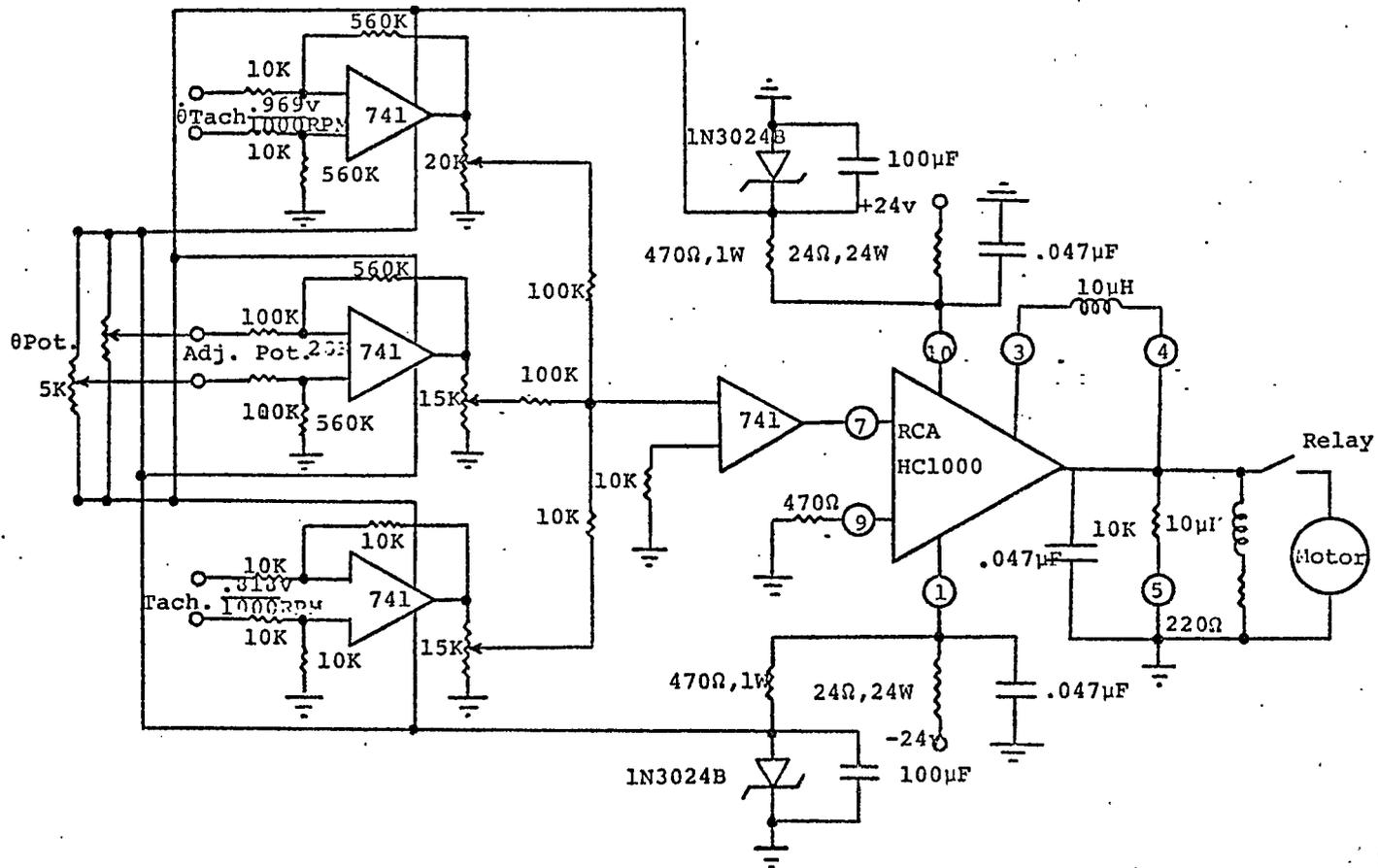
Figure 12. Electronic Circuit of the Inverted Pendulum System
