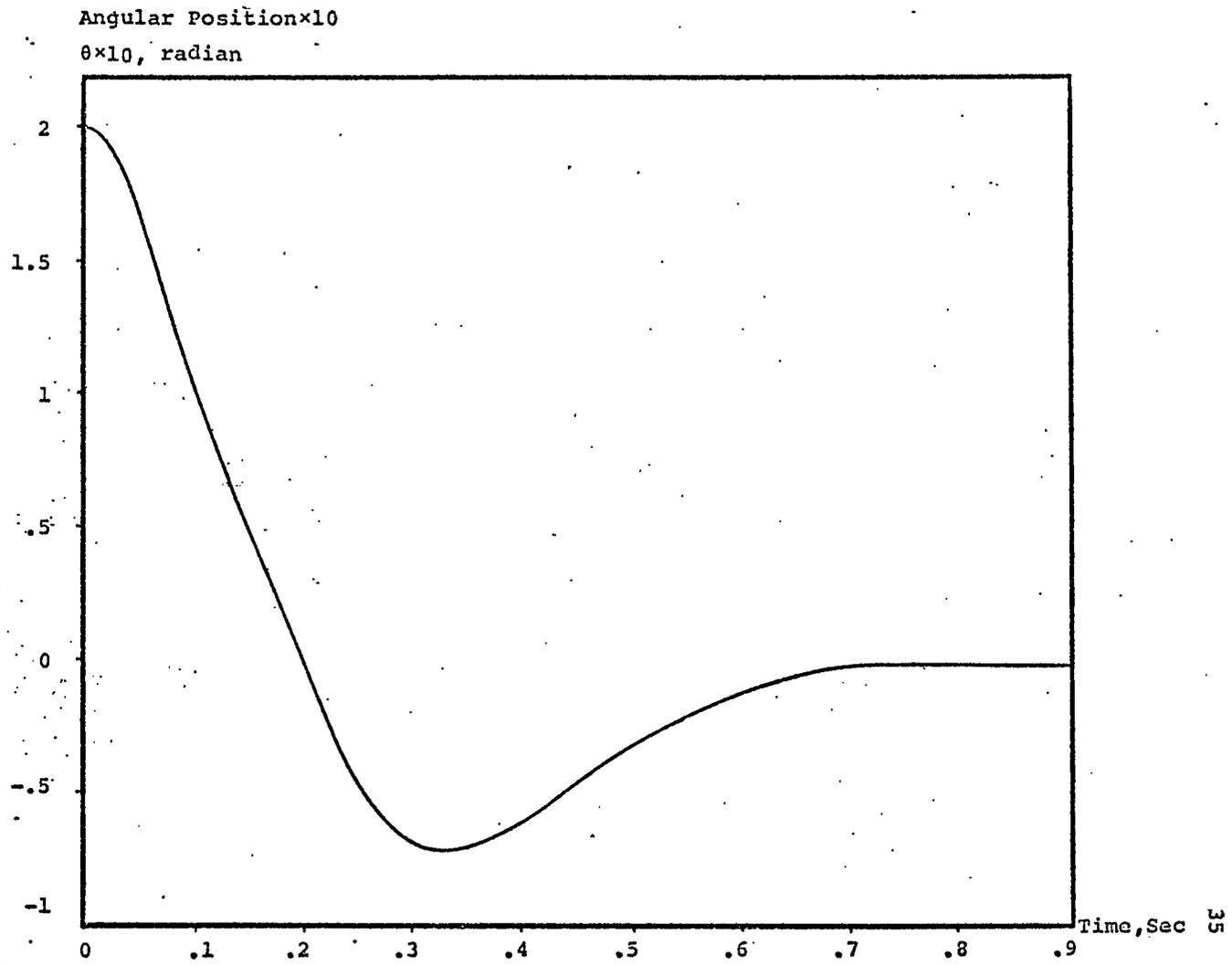
Figure 9.. Zero Input Response of the Angular Position For an Initial Angular Position of .2 Radians
