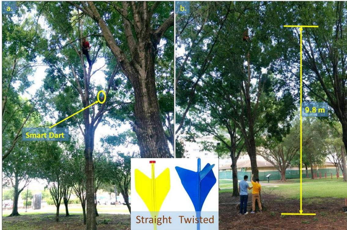
Fig.26: Outdoor Drop test is comparing straight vs. twisted fins performance. a.) dropping a SeismicDart b.) measuring drop height
