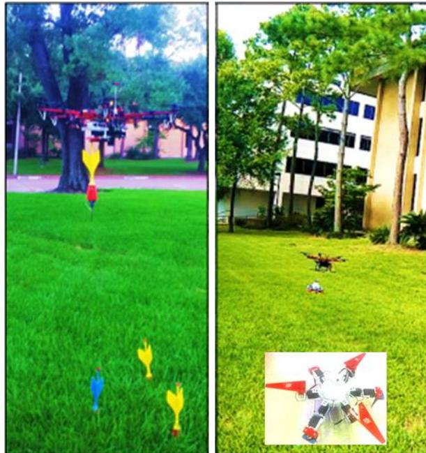
Fig. 2: The heterogeneous sensor system presented in this thesis, a wireless SeismicDarts and a SeismicSpider, both designed for deployment from a UAV.
