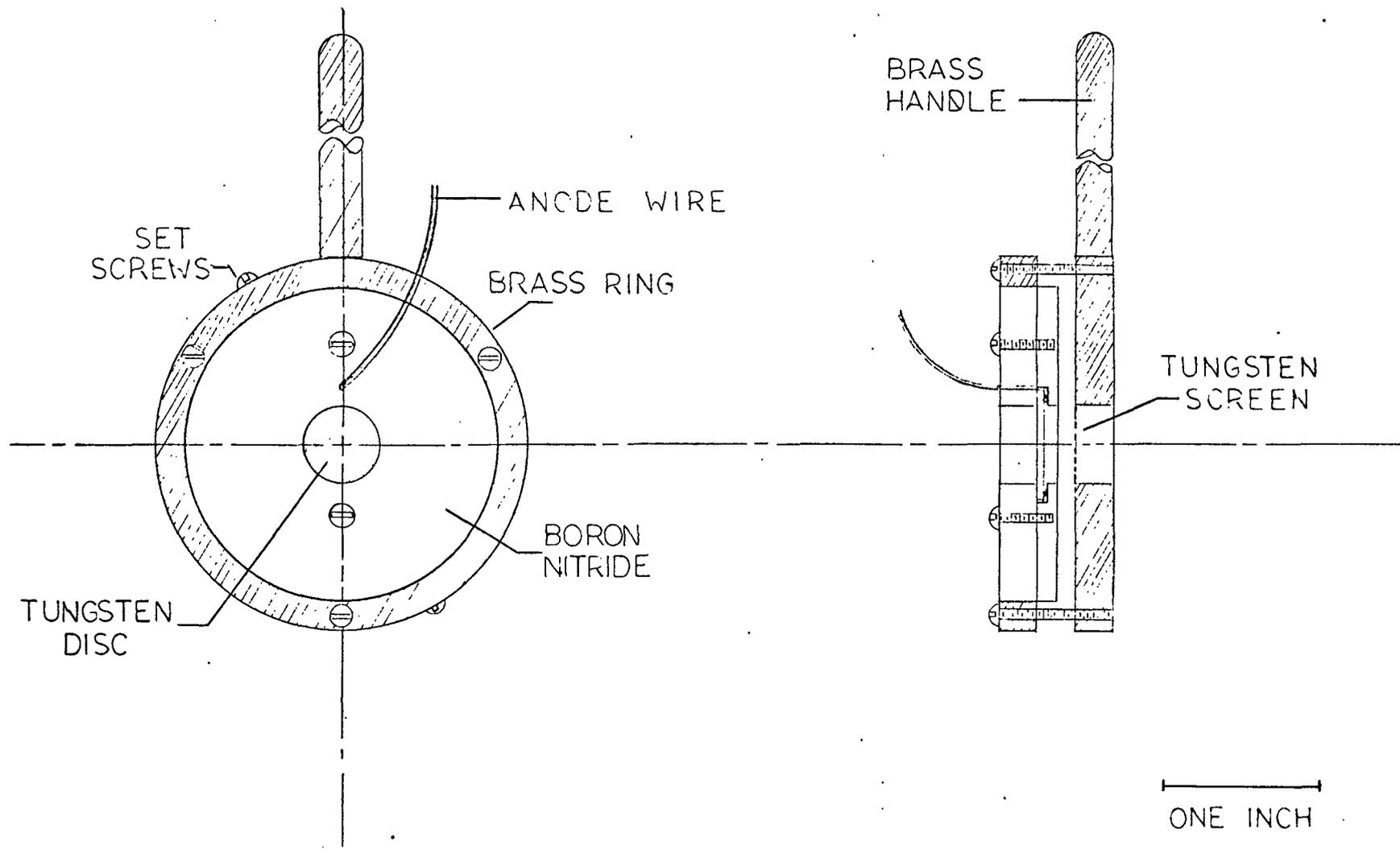
ELECTRON-BEAM HEATED ELECTRON GUN
