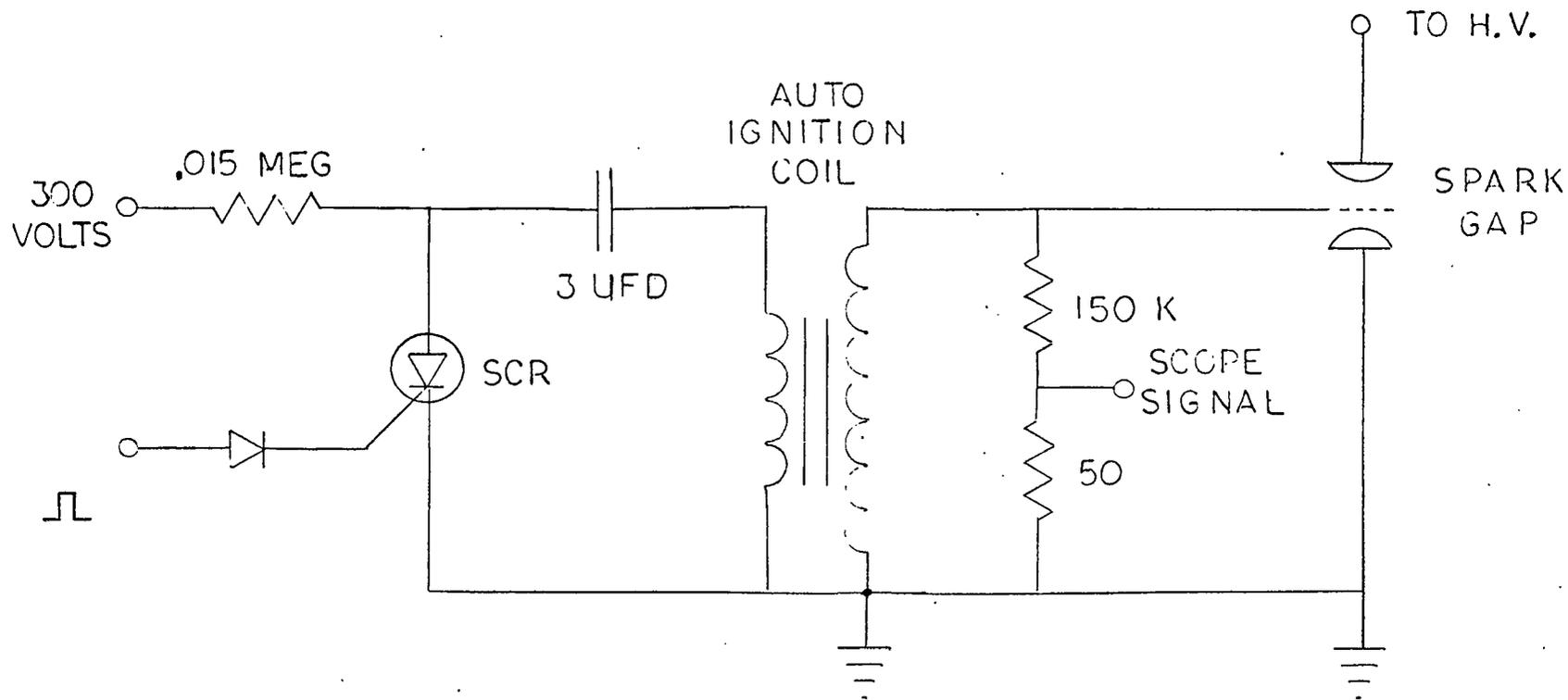
SCHEMATIC OF SPARK GAP TRIGGER UNIT
