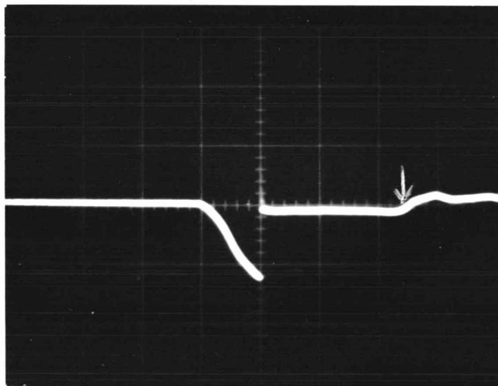
(b) TRIGGER SIGNAL WITH SPARK GAP CONNECTED
