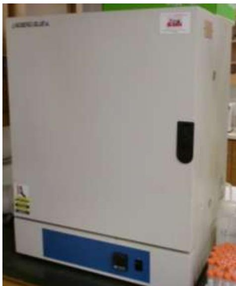
Figure 2.6. Temperature-control oven used for acid digestion
