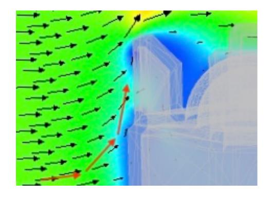
The red arrows show an issue with having a body-tower offset. The upward airflow from the body limits the amount of air entering into the window. To solve this issue the body-tower offset was removed and a lip was added:
