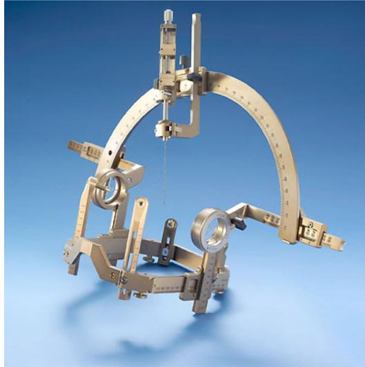
Figure 2.4: Stereotactic frame by Leksell (Leksell Stereotactic System). It includes a three-dimensional reference system and a center-of-arc instrument positioning system, used to as a guide for the insertion of exploratory microelectrodes and final macroelectrodes leads. Reproduced from <http://www.elekt.com/>.
