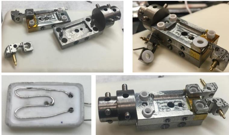
Engagement and disengagement of the electrical pins and the cold finger copper connections.
