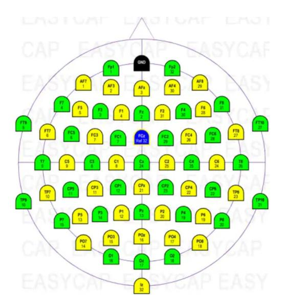
*EEG CAP: Standard 64ch-ACTICAP-slim with built-in electrodes*. DigitalOne. (n.d.). Retrieved July 2, 2022, from https://www.brainlatam.com/manufacturers/brain-products/eeg-cap-standard-64ch-acticap-slim-with-built-in-electrodes-205
