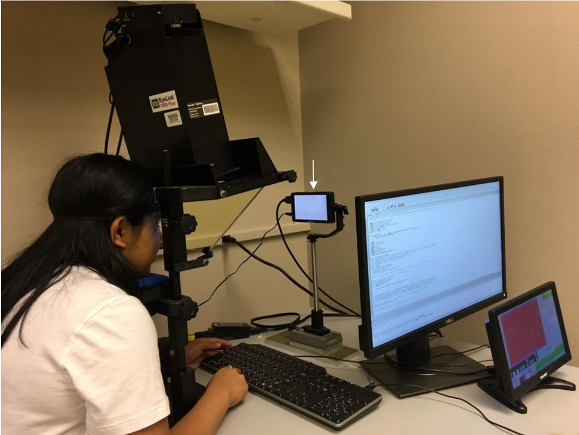
Figure 3.1 The experimental set up for measuring word recognition ability at 40cm. The subject's task is to read the word presented on a miniature monitor display (indicated by the arrow). The subject had the ability to control the pace of the task, as word presentation speed was controlled via the subject keying of the space bar.
