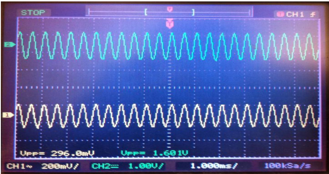
Figure 7.12. AGC output for 1 KHz signal for 1.6Vpp signal
