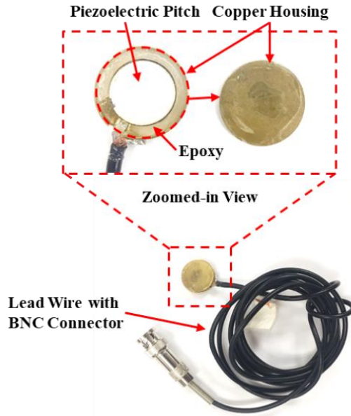
Figure 6-2 Configuration of an enabled PZT transducer assembly
