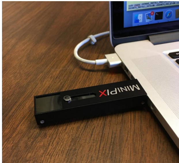
Figure 2.3.1: Image of the MiniPIX plugged into the USB port of a computer.
