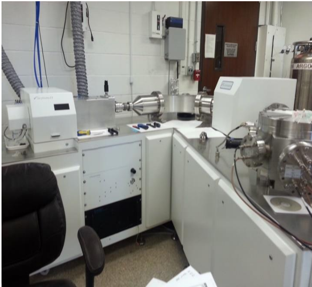
Figure 3.8.2: Nu Plasma II MC-ICP-MS- University of Houston
