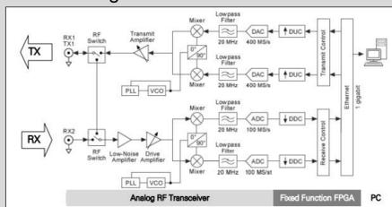
**Figure 1: Block Diagram of the USRP**
