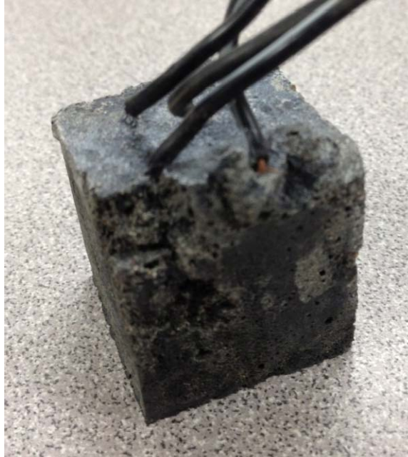
Fig. 3.11 Severe Damage in CNFA Containing 1.75% CNFs by Weight of Cement due to Clumping Before Testing
