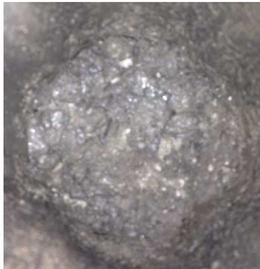
Fig. 3.24 Mortar Mixture After Second Mixing of Step 6, Dough Stage
