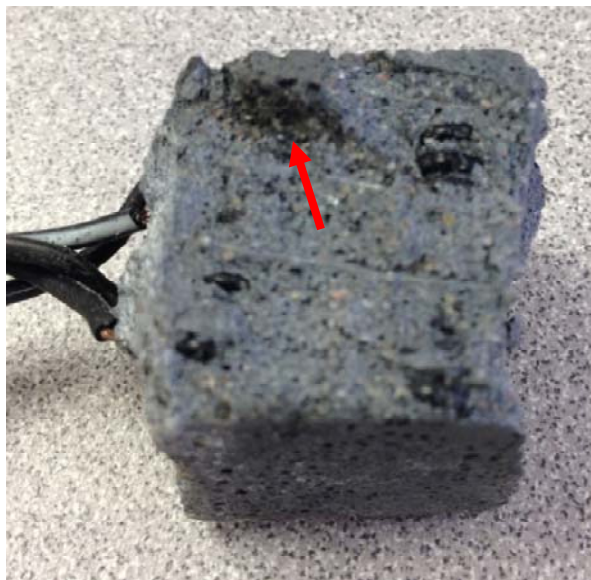
Fig. 3.12 CNF Clump in Tested CNFA Containing 1.00% CNFs by Weight of Cement
