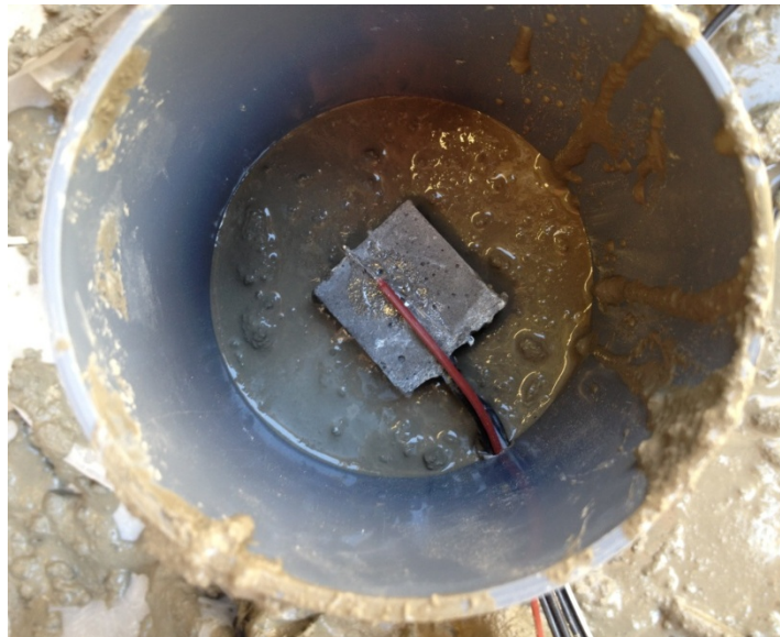
Fig. 6.2 CNFA and Thermocouple in Fresh SCC
