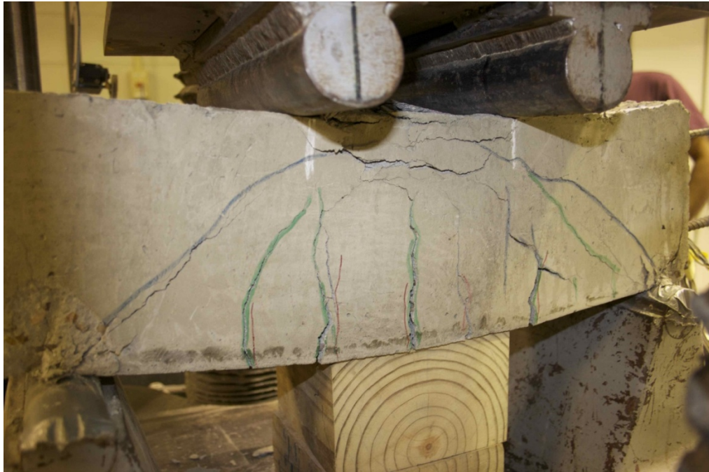
Fig. 7.10 Previously Tested Beam with Flexural and Crushing Failure Modes
