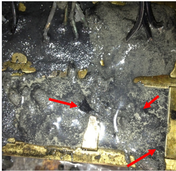
Fig. 3.10 CNF Clumps in Mortar Containing 1.75% CNFs by Weight of Cement
