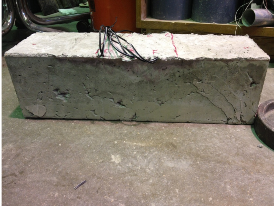
Fig. 7.11 Tested Beam with Shear Failure Mode
