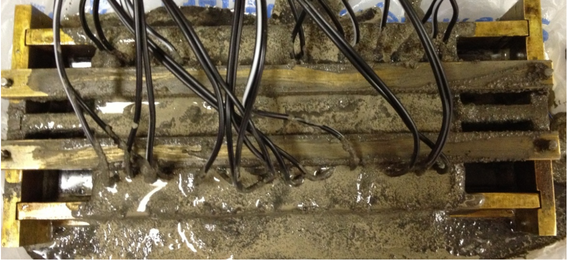
Fig. 3.28 Fresh Mortar Poured into CNFA Formwork
