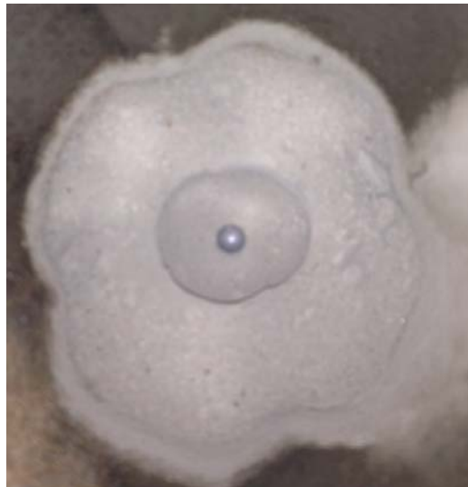
Fig. 3.20 Cement and Sand after Second Dry Mix
