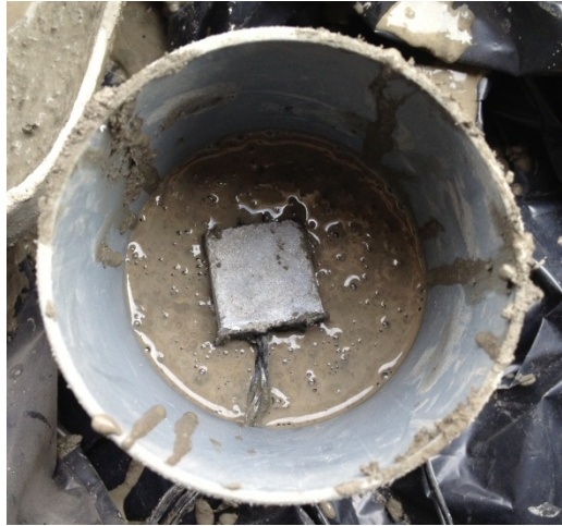
Fig. 5.2 Uncoated CNFA in Fresh SCC
