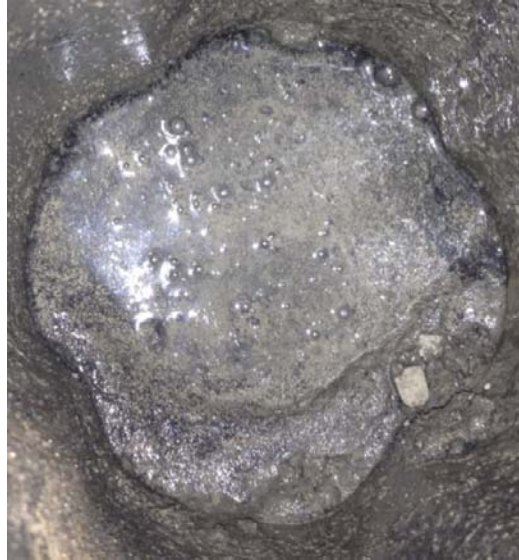
Fig. 3.25 Mortar Mixture After First Mixing of Step 7
