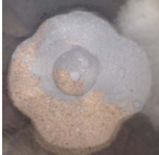
Fig. 3.19 Sand and Cement after First Dry Mix
