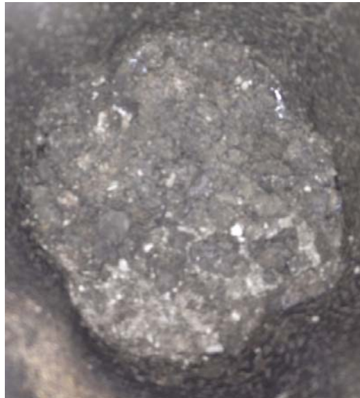
Fig. 3.22 Mortar Mixture after Second Mixing of Step 5, Wet Granulated Sugar Stage
