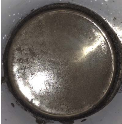
Fig. 3.18 Water, HRWR, and CNF Mixture
