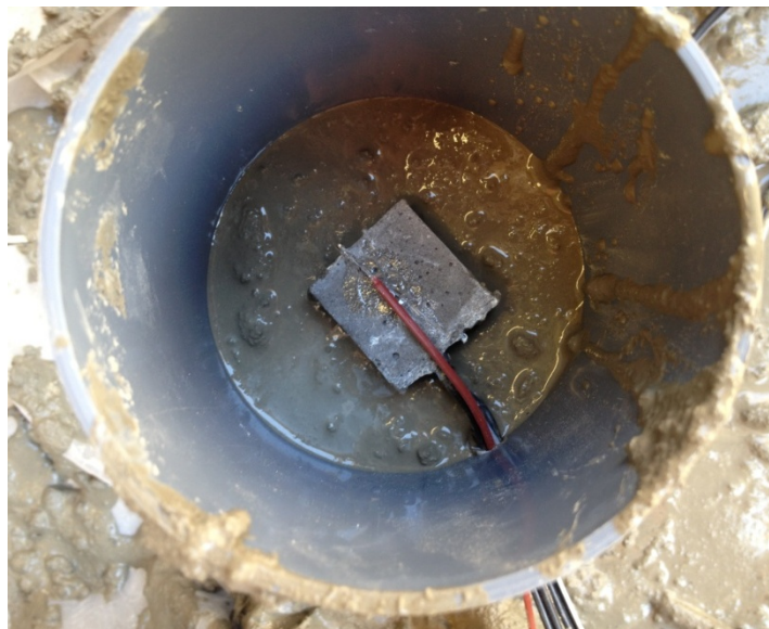
Fig. 5.14 Uncoated CNFA and Thermocouple in Fresh SCC
