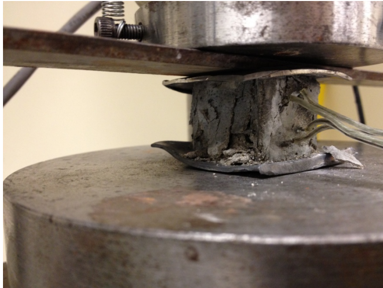
Fig. 3.14 Tested CNFA in Compression
