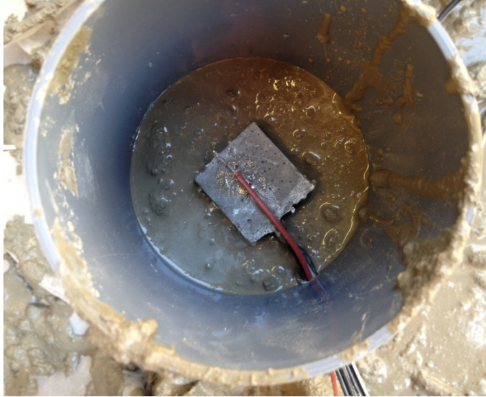
Fig. 4.2 CNFA and Thermocouple in Fresh SCC
