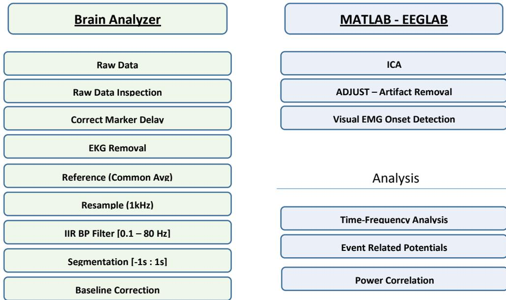
Figure 4: EEG Data Analysis Pipeline
