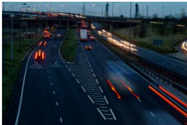
Figure 1.1. Motion blur and moving ghost problems. Note that the vehicles closer to the camera have ghost-like appearances and the spatial extents of their motion blur are larger compared to those far away from the camera. Reproduced from Free-photo.com.
