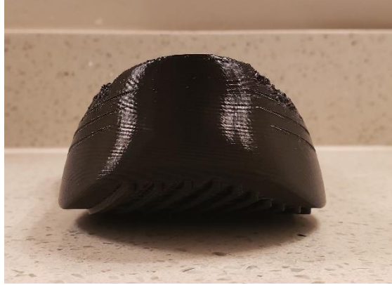
Fig. 60: Sole of the second prototype with a wider heel.
