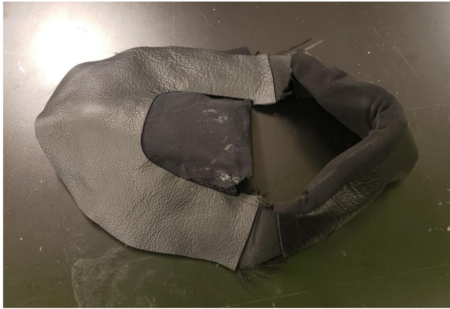
Fig. 43: Glued and sewn upper materials of the first prototype.
