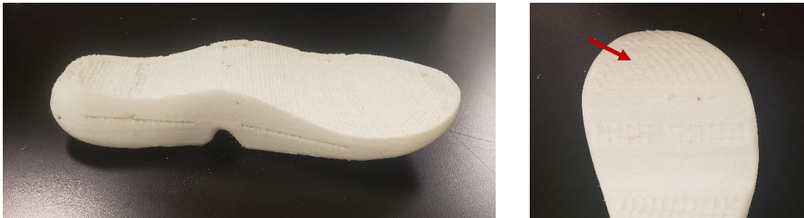
Fig. 42: 3D-printed first prototype sole. The grooves for traction are pointed out in the picture on the right.
