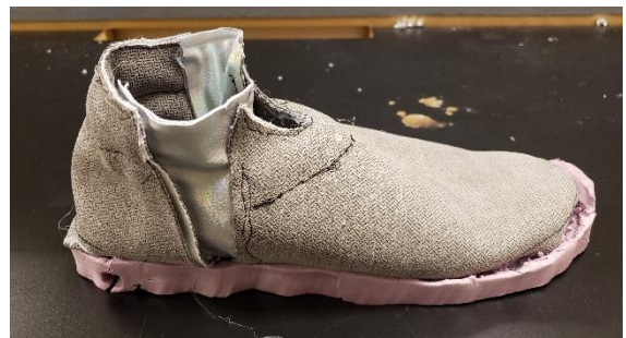
Fig. 34: First fully assembled practice shoe with foam board sole
