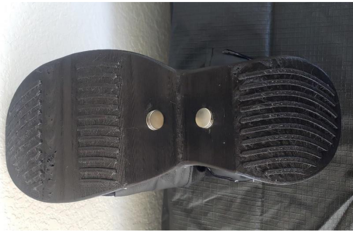
Fig. 68: The second working prototype. Magnets within the sole serve as the bending mechanism.
