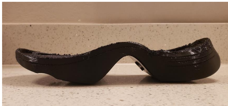
Fig. 59: 3D-printed sole of the second prototype.
