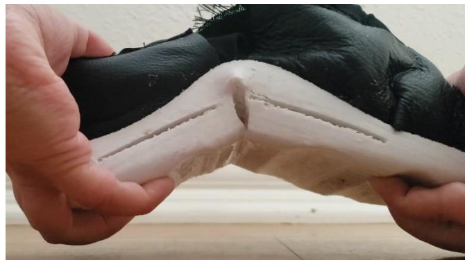
Fig. 46: The bending mechanism of the first prototype.
