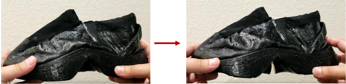
Fig. 85: Successful slip-on method with strong magnets that allow the shoe to stay bent.
