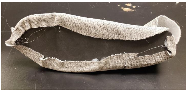
Fig. 33: Upper materials attached to EVA foam insole
