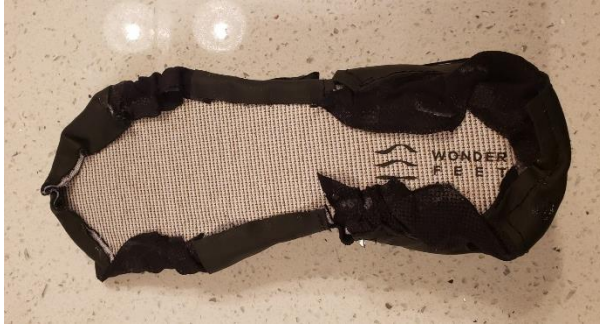
Fig. 64: The upper materials of the second prototype attached to the insole.
