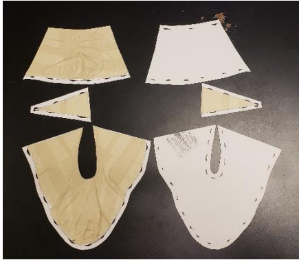
Fig. 31: Masking tape on poster board cut out to use as stencils to cut out fabric
