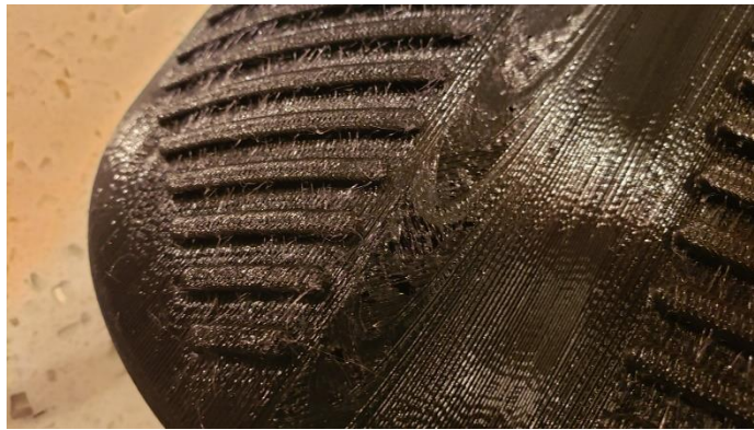
Fig. 61: Sole of the second prototype with deeper grooves for traction.
