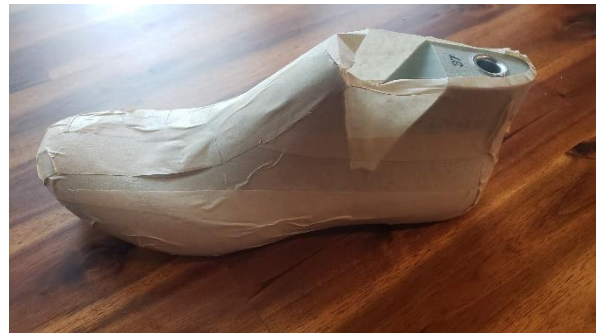
Fig. 30: Shoe last wrapped with masking tape
