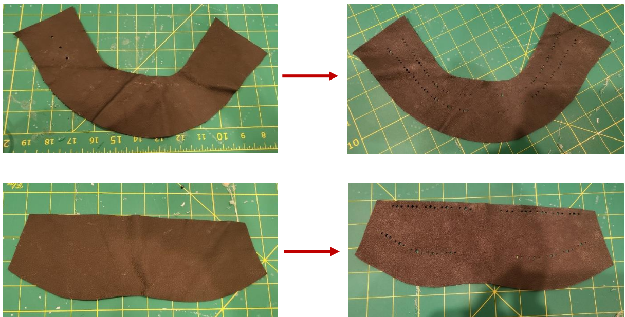
Fig. 79: Punched holes in the leather for breathability
