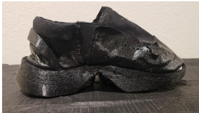
Fig. 81: Fully assembled final design. Fabric stiffener made the upper materials stay up and be able to conform to the foot better.
