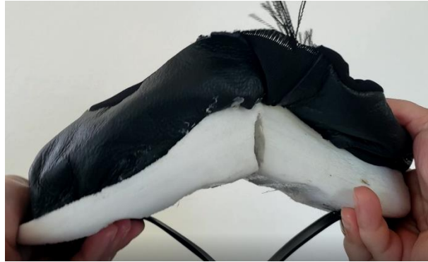
Fig. 56: First prototype with slap-wrist bracelet bending mechanism.
