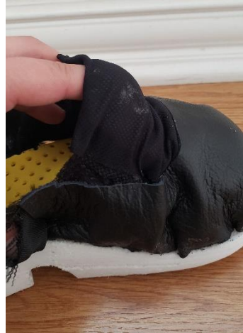
Fig. 45: The stretchable materials of the upper part of the first prototype. This will accommodate for swelling.
