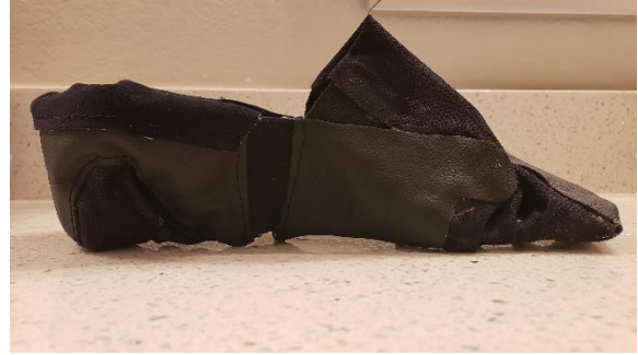
Fig. 64: The upper materials of the second prototype attached to the insole.
