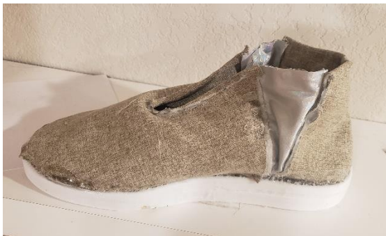
Fig. 35: Second fully assembled practice shoe with 3D-printed TPU sole
