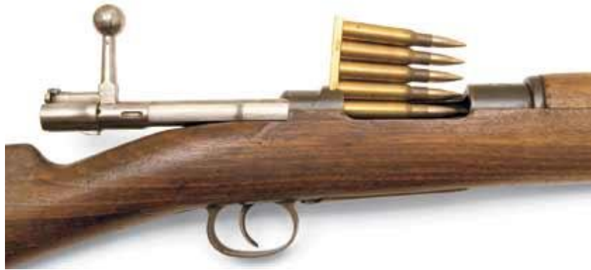
Figure 37: a 7mm Mauser with its five-round clip. To load, the soldier positioned the full clip in the bolt holder, then pushed all five cartridges in at once with the thumb. 209
