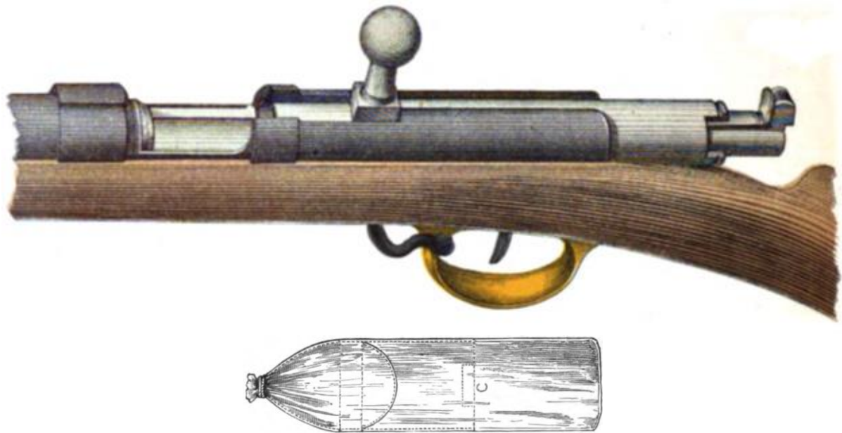
Figure 6: The Dreyse needle-fire and its cartridge. The latter contained its primer at "C", requiring the needle-like firing pin to pierce the base of the cartridge and travel through the powder charge. Ignition consumed the entire cartridge. 54
