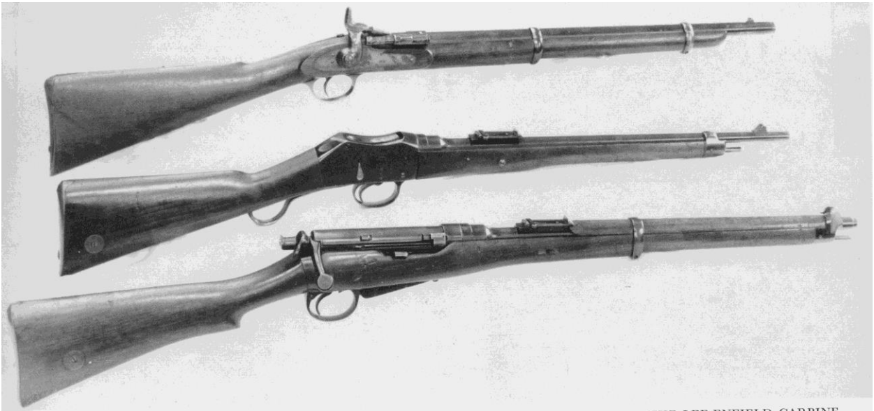
Figure 39: British cavalry carbines. Top is the Snider; middle, a Martini-Enfield (a single-shot Martini action married to a .303 Enfield barrel) and bottom is the Lee-Enfield. Both lower weapons saw service in the Second Boer War. 217
