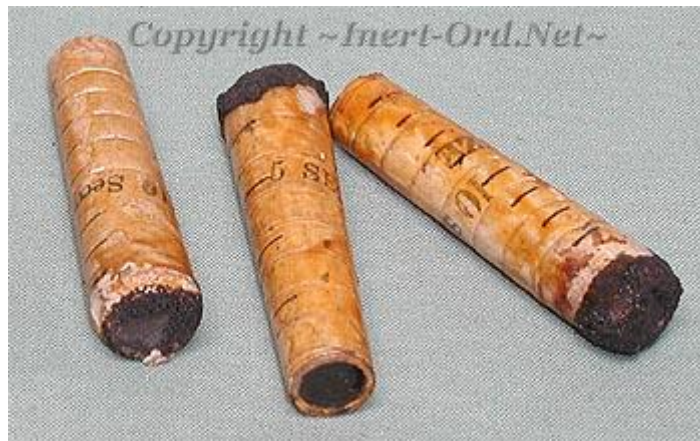
Figure 9: Examples of American Civil War era time fuzes showing the unsupported powder column at the bottom. 95
