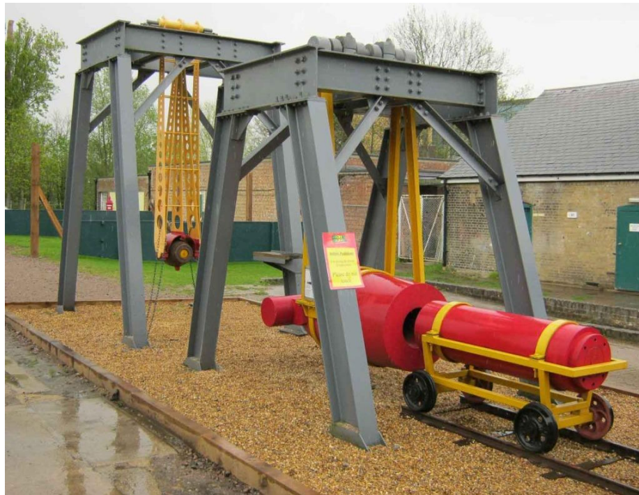
Figure 20: A ballistic pendulum for testing powder and explosives at the Royal Gunpowder Mills, Waltham Abbey, Essex. Behind it is a smaller ballistic mortar, used for the same purpose. The frames are of modern construction. 162
