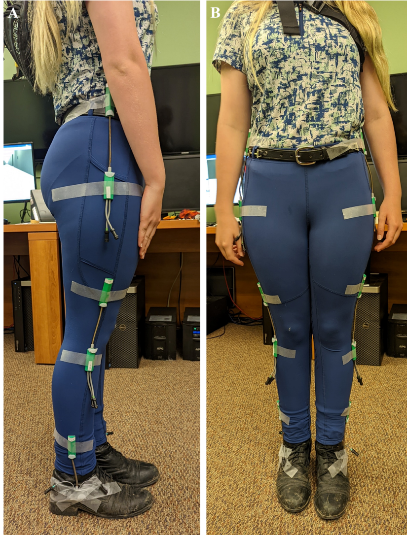
Figure 5: (A) Sagittal and (B) frontal view of the goniometers (Biometrics Ltd, UK) placed on the subject's hip, knee, and ankle joints. The joint centers were found through palpitation, and held in place through tape.
