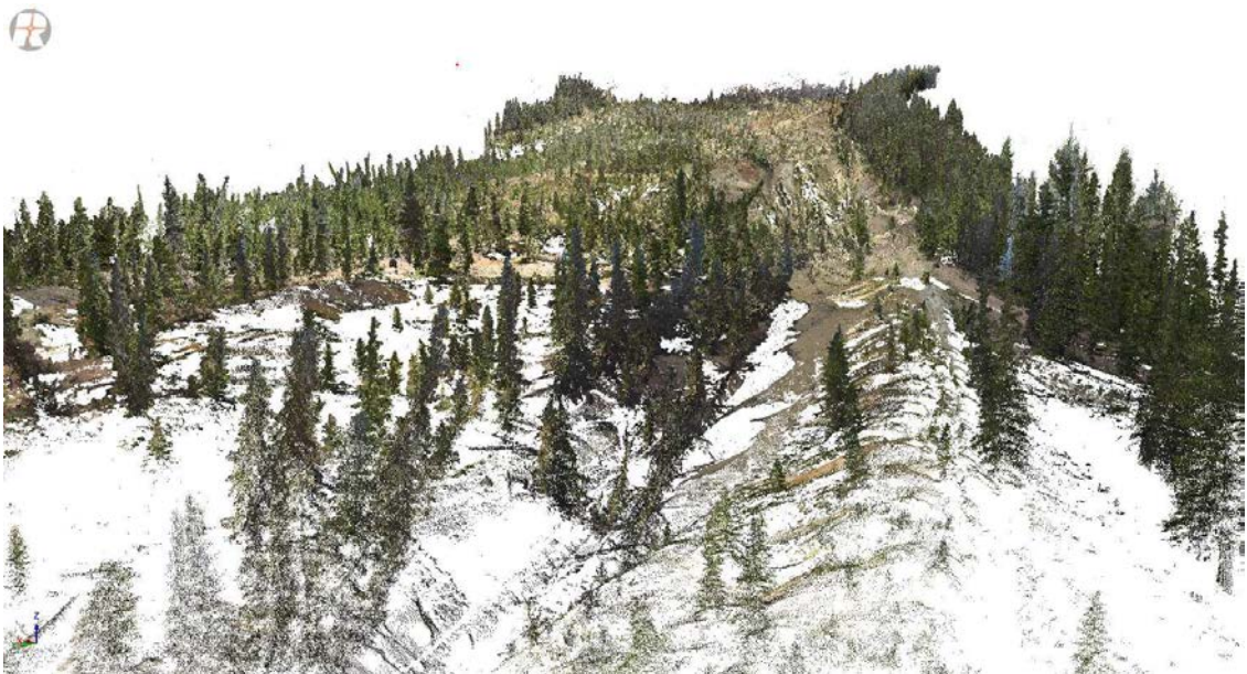
Figure 2-12 TLS registration results colored by images taken by the camera collocated with the scanner.
