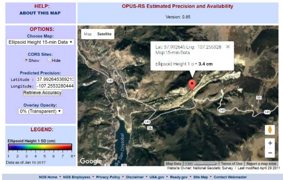
Figure 2-8 Horizontal and vertical components accuracy of OPUS-RS results at the Slumgullion landslide. Horizontal accuracy (top) is below 1 cm for one sigma. Vertical accuracy (bottom) is below 3.5 cm for one sigma.
