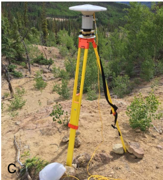
Figure 1-8 Field setup of GPS units. (a) a Trimble NetR9 GPS unit associated with a TLS big cylinder reflector; (b) a Trimble R10 GPS unit associated with a TLS small cylinder reflector; (c) a Trimble NetR9 GPS unit associated with a TLS small cylinder; the plastic bag on the ground contains the receiver and the yellow cable is the TNC antenna cable; (d) the adapter between the antenna and reflector.
