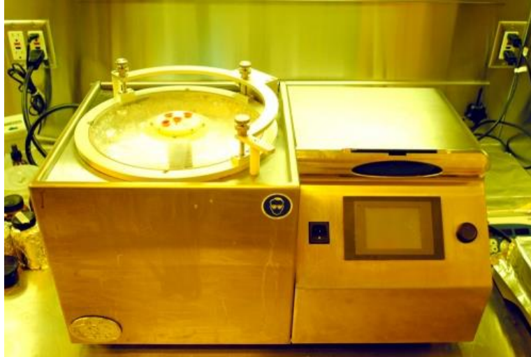
Figure 9.5 Brewer Cee 200 spin coater in UH nanofabrication facility.
