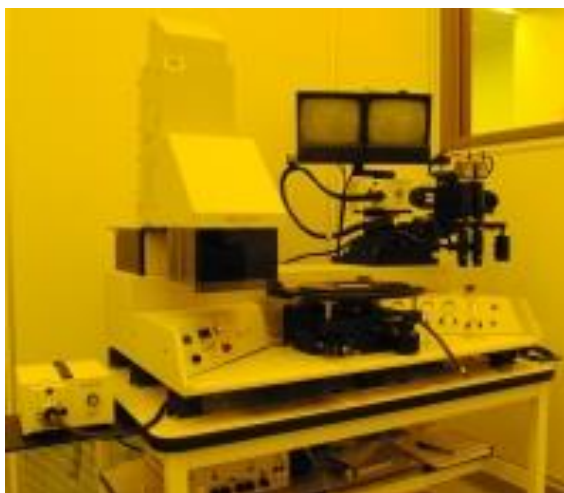
Figure 9.6 Kasper mask aligner in UH nanofabrication facility.
