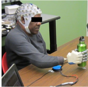
Figure 3.1 Experimental setup. Amputee participants were fitted with the IH2 Azurra robotic hand to their residual limb sockets. Sixty-four channel active EEG was recorded simultaneously while participants performed the grasping task.
